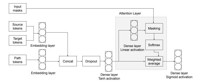
Figure 2: The neural network architecture to identify mistakes in boundary conditions.
